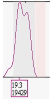
Figure 2: A configuration which inaccurately accepts broad peak width can result in mischaracterization of heterozygous loci.
